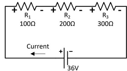
$R_{TOTAL}$  or  $R_T$  represents the *equivalent* or *total* resistance of all the resistors in a circuit. For resistors in series;  $R_T = R_1 + R_2 + R_3 \dots + R_n$
